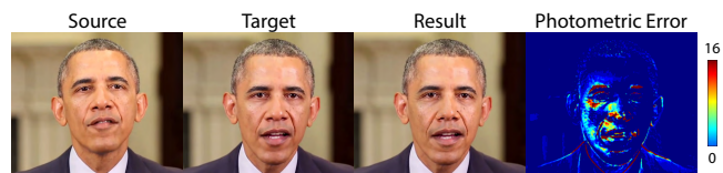
Figure 9: The photometric error of a self-swapping in which we use the first frame as the source image. Image courtesy: The White House (public domain).
